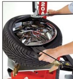
*High-performance mount/demount head with tire iron slot designed to provide extra assistance and increase versatility.*
