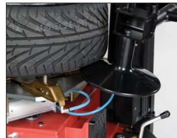
*Locking roller disc lifts and removes bottom bead effortlessly and securely.*
