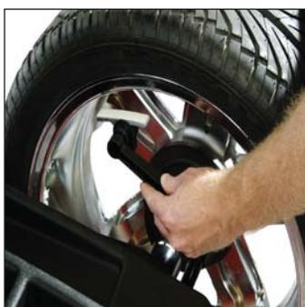
Accu-stik parameter entry arm holds the weight while the screen shows the technician where to place it
