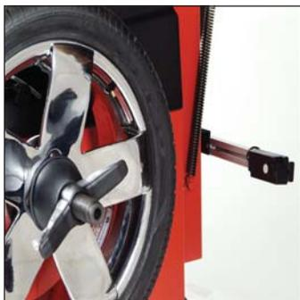
Automatic run-out system tests every wheel for run-out and eccentricity
